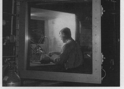
CLIMATIC EXPOSURE chamber is readied for tests which will subject unit to high altitude, high temperatures, and high humidity. Shown here is Glenn Morehouse, 1611, preparing instrumentation on test unit. Other climatic tests in the Test Laboratory can create fogs, salt mists, dew, below sea level atmospheric pressures, sunshine, rain fall!
